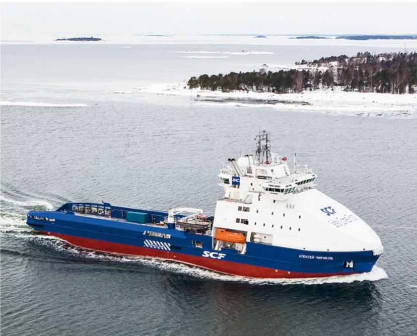
vrability even in the most difficult ice conditions. For manoeuvring and position keeping, two bow tunnel thrusters are provided.
